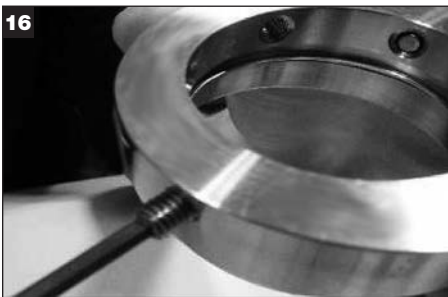
IMPORTANT: The set screws should not protrude into the inner diameter of the lock ring prior to installing onto the seal sleeve.
