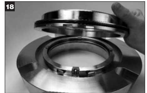
Remove the adapter from the gland. Remove the adapter O-Ring (Z) and discard. Set the adapter aside.
