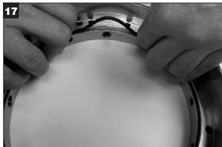
Apply a thin film of grease to the lock ring O-Ring (Y) and insert it into the inside diameter groove in the lock ring.
