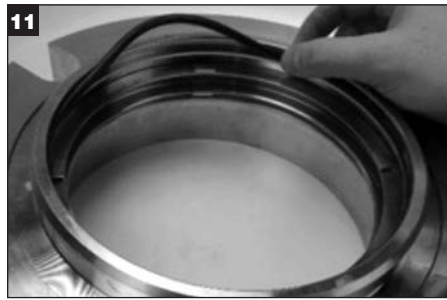
Apply a thin film of grease to the stationary O-Ring (X) and install in the inside diameter groove in the adapter.
